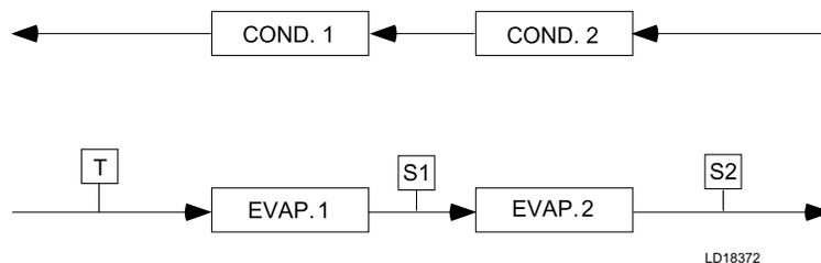
**S** – Temperature Sensor for Chiller Capacity Control
