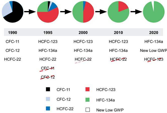
FIGURE 1 - USE OF HFC-134A IN CENTRIFUGAL CHILLERS
