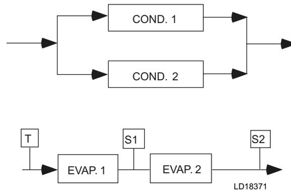
**FIGURE 16 - SERIES EVAPORATORS PARALLEL CONDENSERS**
