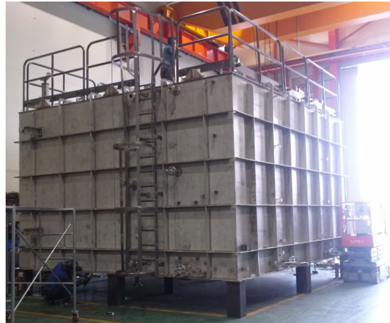
Foam Tank (110m 3 ) for Egina FPSO
