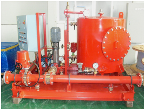
Helidack Foam Skid : Helicopter Deck
